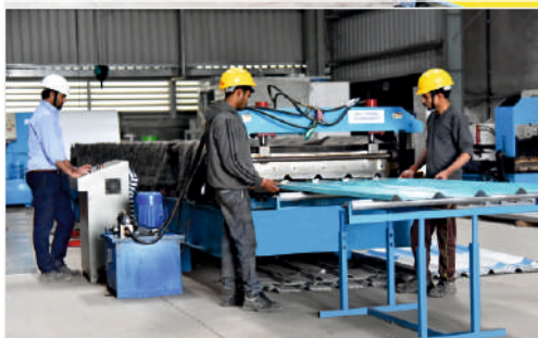
ROOF & SIDE SHEETING MACHINE
